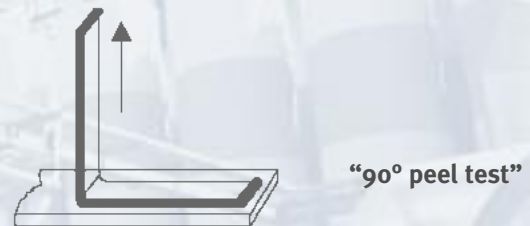
Bonding Aluminium to glass: 90° peel
